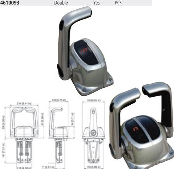
Double action control for inboard, outboard and stern drive engines throttle #ULTRAFLEX and shift control. Available with or without trim. Uses directly C14 / MACH14 cables or C2 / C8 / MACHZero cables with included K59 kit. C5 / C16 / MACH5 cables can be connected with K60 kit. C22 cable can be connected with K61 kit. C36 / MACH36 cables can be connected with K62 kit. With optional X12  $\,$ safety switch (4620112) engine can be started only with disengaged gearbox.
